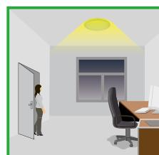
With insufficient natural light, the sensor switches on the light automatically when person enters room.
