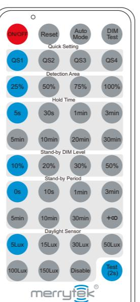
The green work light of microwave sensor will flash 3 times if set successfully by remote control.
