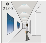
1 The light switches on at 100% when there is movement detected.
