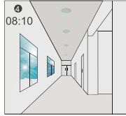
5 The light automatically turns on at 10% when natural light is insufficient (no motion).
